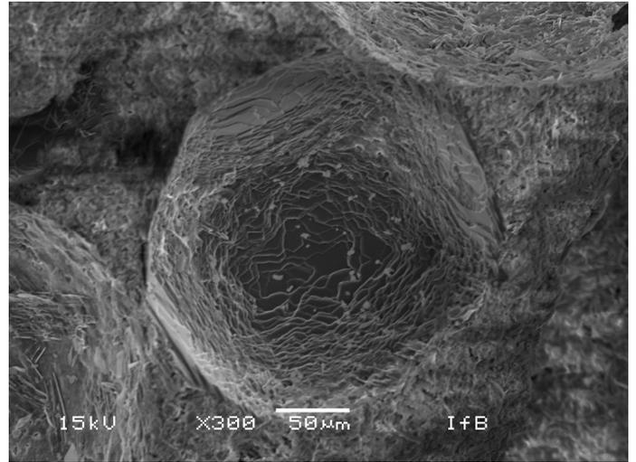
Figure 8. SEM-Picture of a pore with platy crystal structures.
