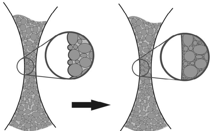
Figure 4. Optimization of the bubble surface using higher water content and silica fume.
