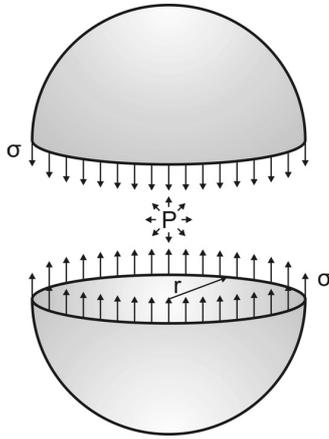
Figure 2. Schematic diagram of a bubble.
