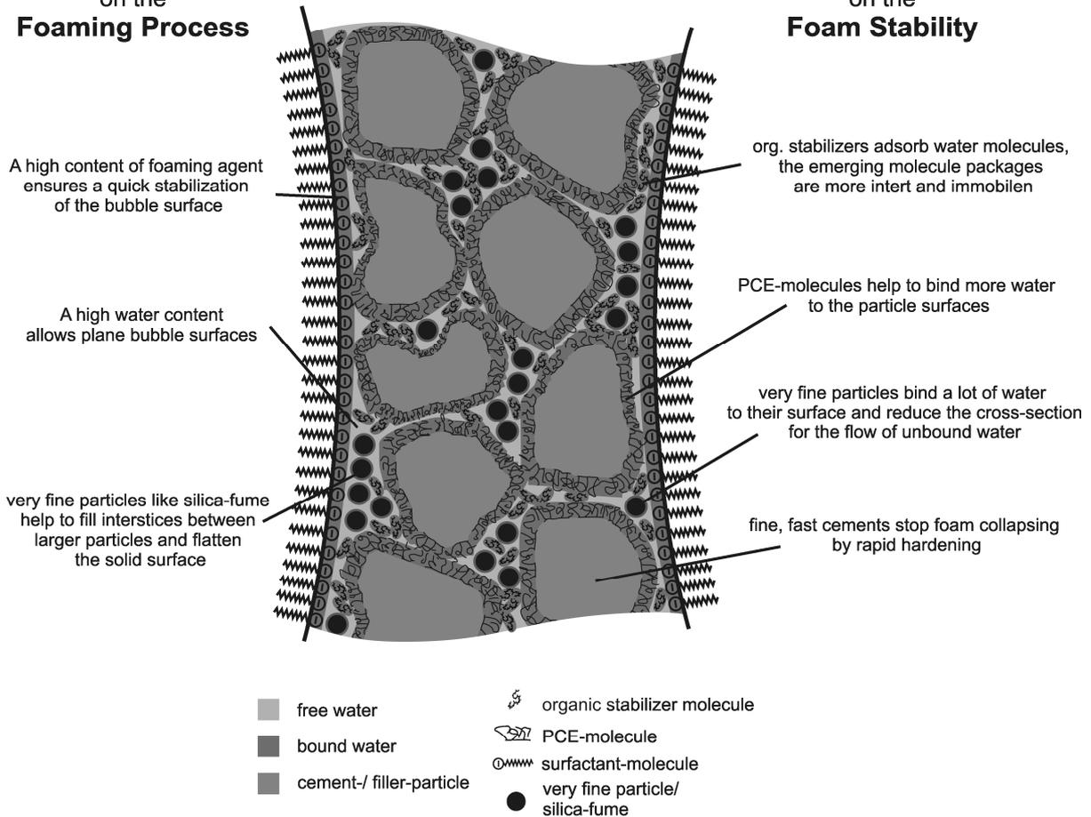
Figure 6. Model of the influences of different components of cement paste on foam processing and foam stability.
