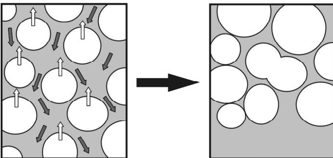
Figure 3. Schematic diagram of drainage and coalescence.
