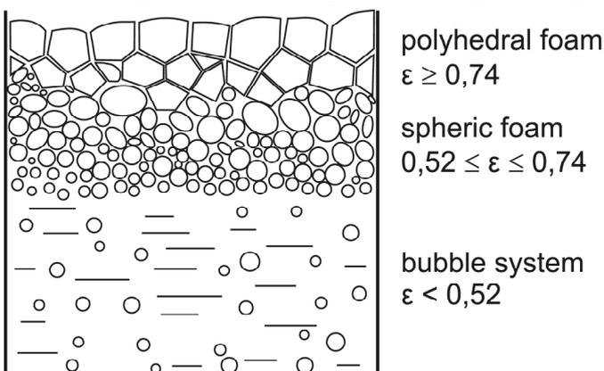
Figure 1. Different types of foam, characterized by the gas content  $\epsilon$ , based on KERN 2002.
